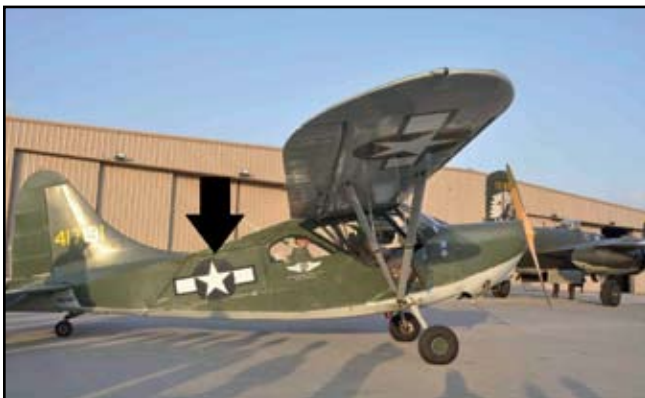
Right side view of the L-5 showing the large hatch of the "B" Model.
