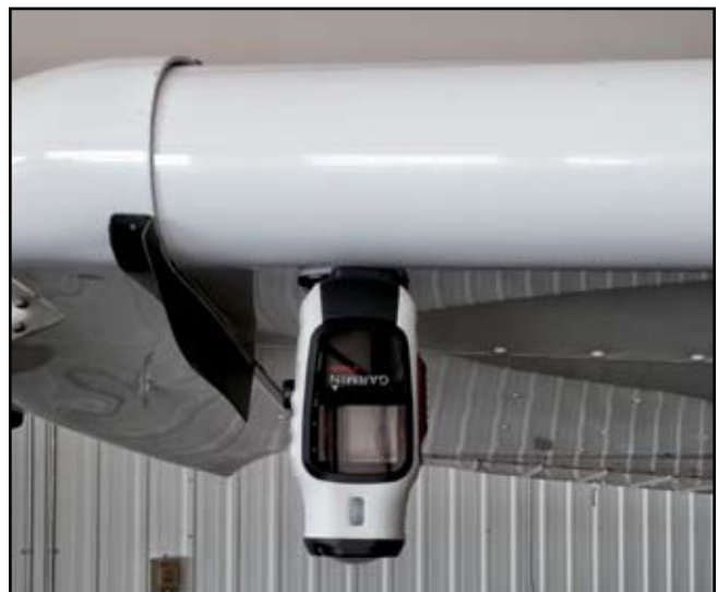
Front view of the VIRB camera mounted near the wingtip on CAP Cessna-182T (N158CP).
