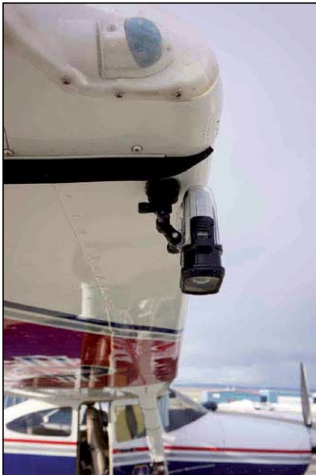
Side view of the VIRB camera mounted near the wingtip on CAP Cessna-182T (N158CP).
