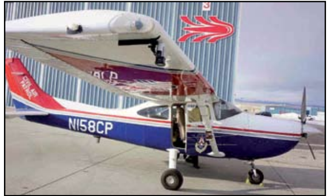
The VIRB camera mounted on the right wing of a South Dakota Wing Cessna-182T.
