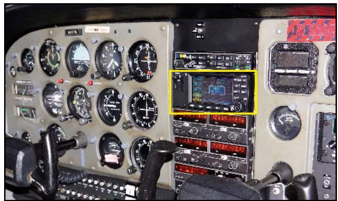
Wide angle view of the aircraft instrument panel showing the placement of the G400W.
