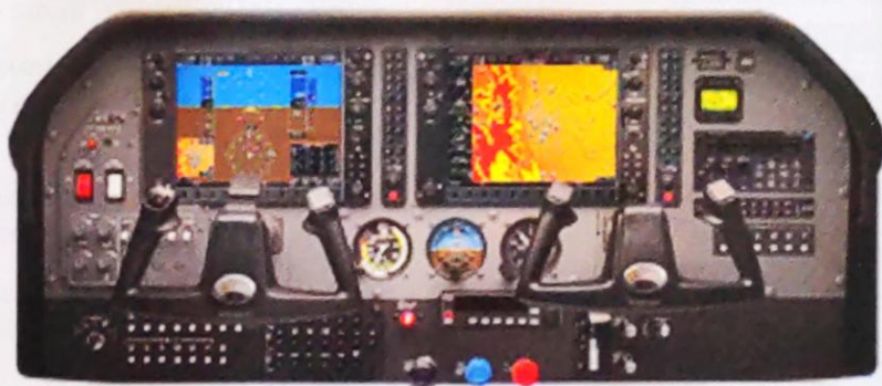
An artist's rendition of Garmin's G1000 glass cockpit. Civil Air Patrol is ordering 40 Cessna C-182 Skylanes and one Cessna C-206 outfitted with the new high-tech cockpit.
